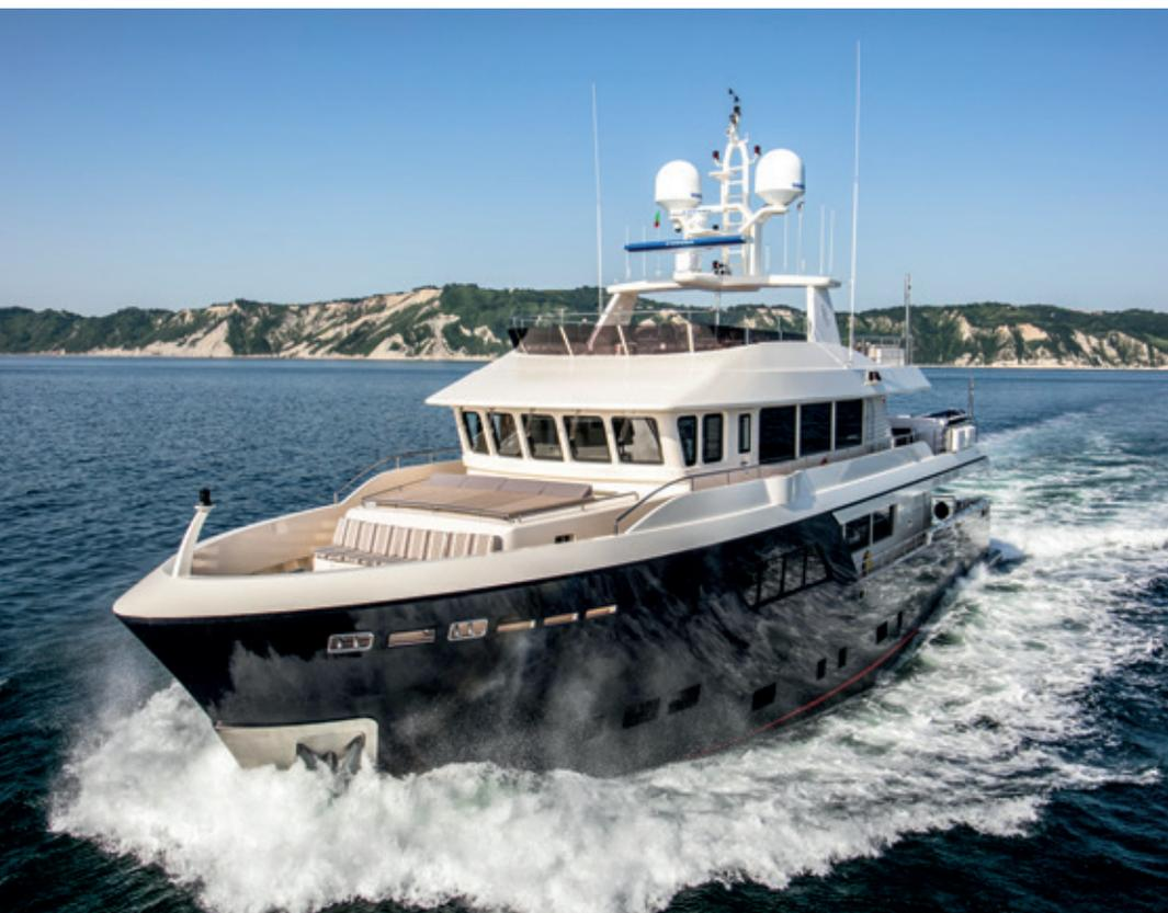
HYDRO TEC HA PROGETTATO PER IL CANTIERE DELLE MARCHE LA FAMIGLIA DI NAVETTE DISLOCANTI IN ACCIAIO DARWIN CLASS, IMBARCAZIONI IN GRADO DI SOLCARE GLI OCEANI SENZA RINUNCIARE AL COMFORT, PERMETTENDO DI TRASCORRERE LUNGHI PERIODI A BORDO.
