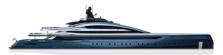
Concept "Crossbow" is a unique take on a 100-metre superyacht, based on an aluminium hull and superstructure, the sleek design has a beam of just 12.5 metres — more than a metre less than average for this size bracket. What's more, the draught has been kept to just 3.5 metres to ensure Crossbow can reach cruising grounds that would normally be off-limits for such large yachts.
